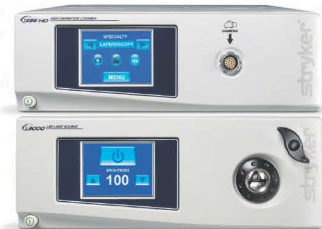
L9000 light source control from 1288 HD head by Firewire Connection
